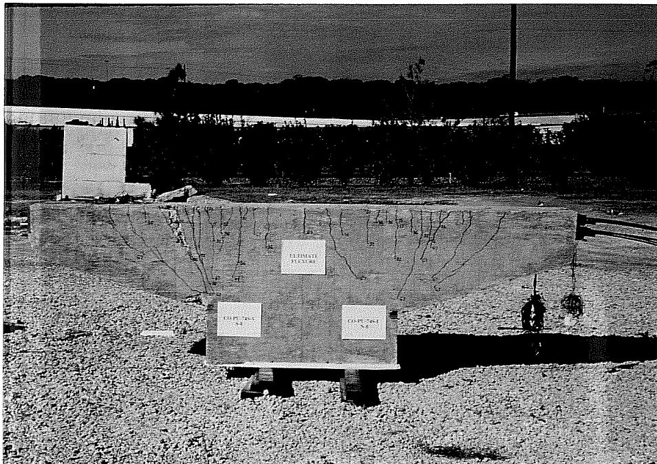
Figure 3.6 CO-PU-74S-I and CO-PU-74S-V Overhangs After Testing
