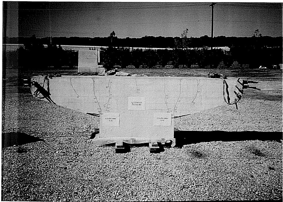
Figure 3.4 CO-PS-100S Overhangs After Testing
